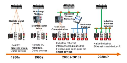
10Mbs Single Twisted Pair Ethernet addresses most Fieldbus applications up to 1200m. Furthermore, many devices require power, and this can also be easily covered by the currently proposed cables the majority of which will be based on a larger conductor size of between 18-24AWG dependent upon distance, and primarily of a screened construction.
